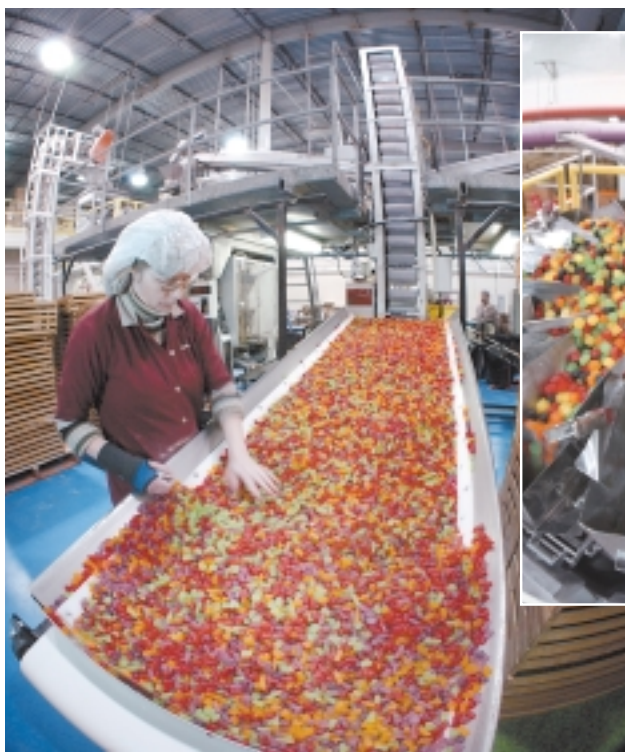
Karen Johnson examines jujubes as they head toward a Hayssen form/fill/seal machine (inset) for packing into large-count cellophane bags.
