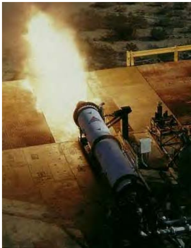
Fig. 1. Test Firing of AMROC H-1500 Motor
