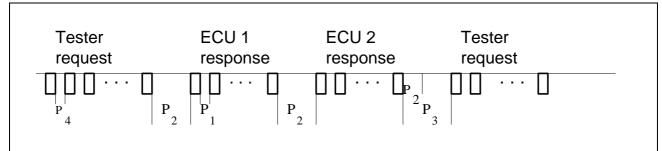
Figure 4 - Message flow, timing
