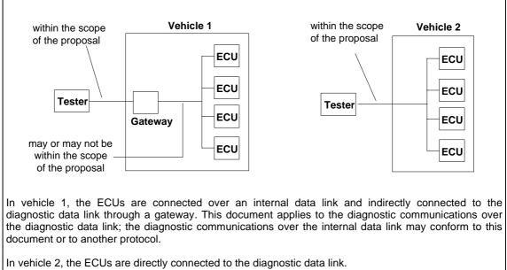
Figure 2 - Vehicle diagnostic architecture
