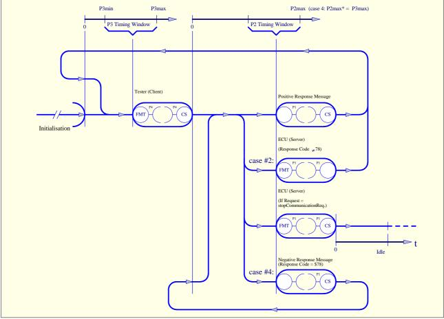
Figure B2.1 - Functional addressing - single positive response message - single server (ECU) addressed
