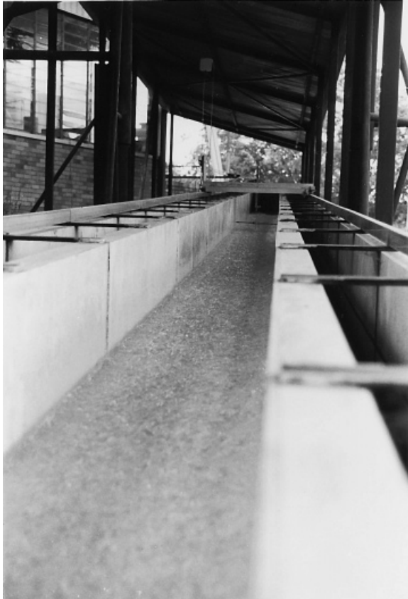
Fig. 2. Photograph of chute flow in operation. Smooth chute flow, Q = 0.075 \text{ m}^3/\text{s} ( 6,480 \text{ m}^3/\text{day} ), \tan\theta = 7\% , b = 0.5 \text{ m} , d \sim 0.035 \text{ m} , V \sim 4.3 \text{ m/s} . View from downstream (flow from top to bottom).
