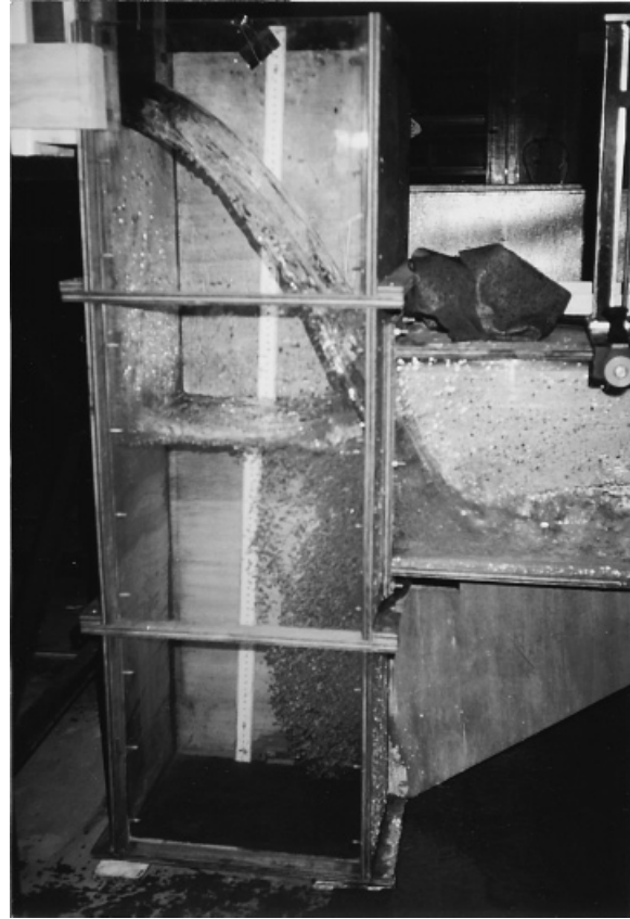
Fig. 17. Photograph of the Recret dropshaft model in operation. Regime R2, Q = 0.000975 \text{ m}^3/\text{s} , h/L = 1.68 , D/L = 0.83 , d_c/L = 0.259 . Side view, flow from left to right. High-speed photograph ( \sim 50 \mu\text{s} ).
