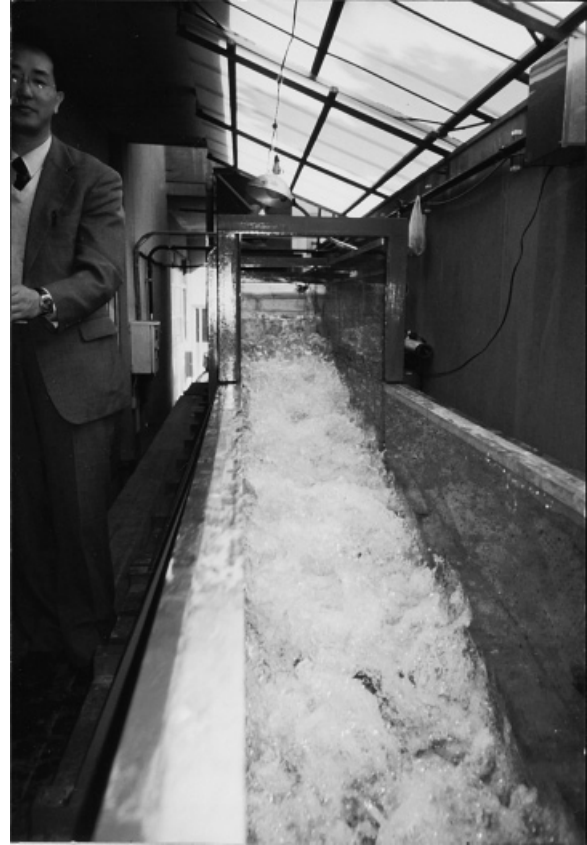
Fig. 3. Photograph of chute flow in operation. Stepped chute flow, Q = 0.033 \text{ m}^3/\text{s} ( 2,850 \text{ m}^3/\text{day} ), \tan\theta = 20\% , h = 0.1 \text{ m} , b = 0.4 \text{ m} . View from downstream (flow from top to bottom).
