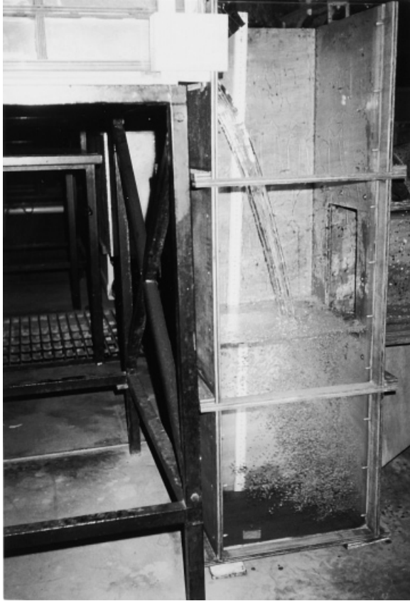
Fig. 16. Photograph of the Recret dropshaft model in operation. Regime R1, Q = 0.00104 \text{ m}^3/\text{s} , h/L = 1.68 , D/L = 0.83 , d_c/L = 0.0582 . Side view. Flow from left to right. High-speed photograph ( \sim 50 \mu\text{s} ).
