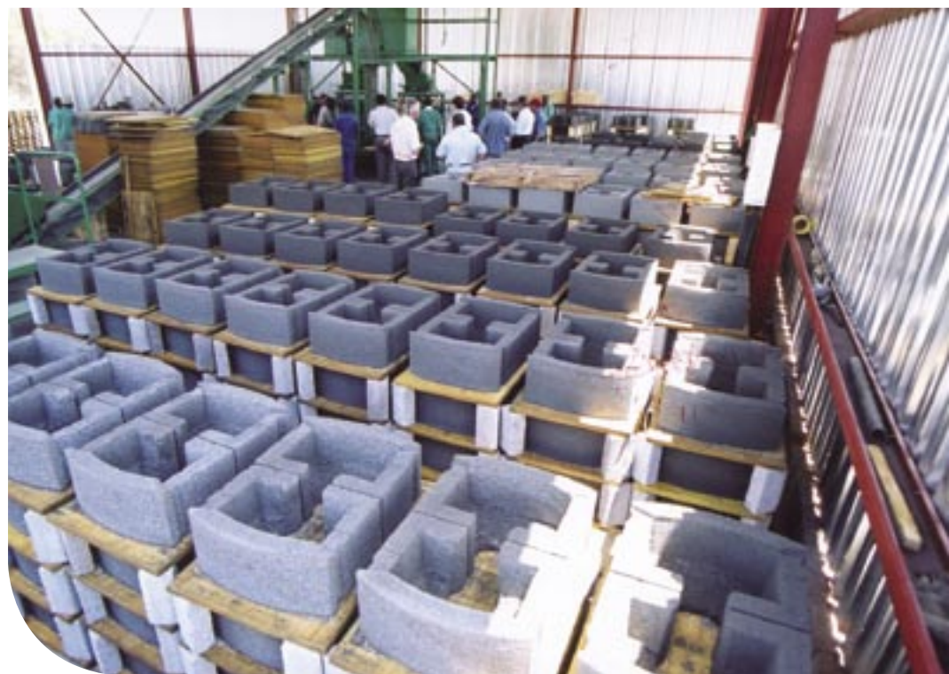
A batch of concrete retaining blocks awaits packing and strapping at the production plant.
