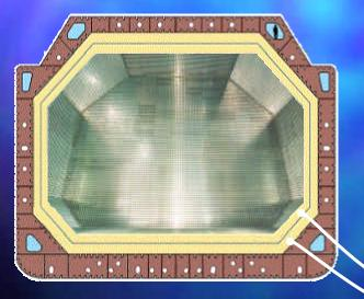
Tank cross section showing dual membrane interior to hull tank
