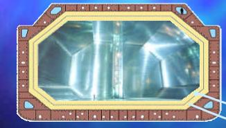
Tank cross section showing dual membrane interior to hull tank
