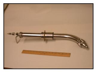
Fig. 15 Photograph of the Two-Fluid Nozzle Assembly.
