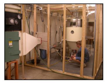
Fig. 14 Photograph of the Spray Drying System Showing the Chamber and HEPA Filtration System.
