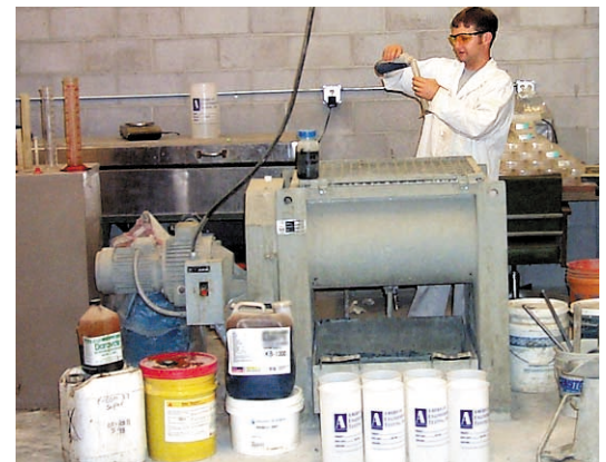
Concrete Specialist Tim Suess measures chemical admixture for trial batching.
