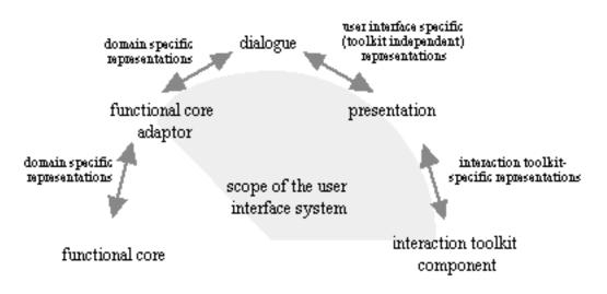
Figure 2.1. The Arch reference model: its components and data representations. Arrows indicate data flow. The shaded arch illustrates the scope of the user interface system.
