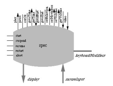
Figure 7.2. Simple Player<sup>™</sup> modelled as a single ADC interactor. Grey lines and arrows represent groups of gates, described by the relevant heading in italic print.
