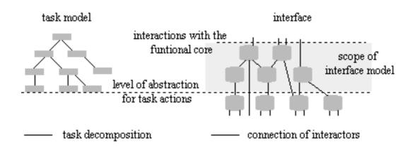
Figure 7.7. Drawing mappings between task and interface models.
