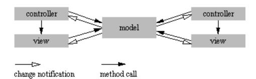
Figure 2.2. The MVC architecture. A model and two view-controller pairs.
