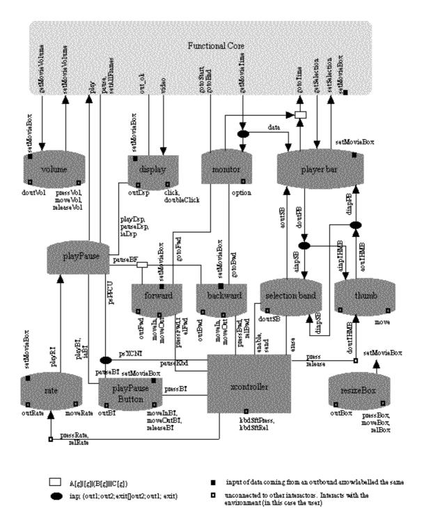
Figure 5.5. Graphical representation of the configuration of ADC interactors which model the Simple Player<sup>TM</sup> interface.
