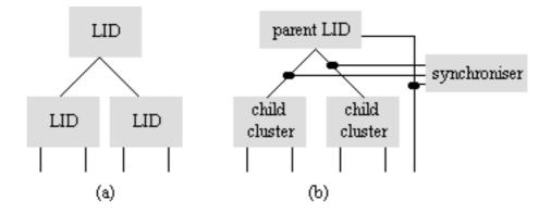
Figure 3.6. (a) Hierarchical composition of LIDs as in [53] and (b) the recursive composition of clusters of [66]. An LID may have many input gates (lines at the bottom side) and a single output gate (lines at the top). Blobs indicate synchronisation of all connected processes.
