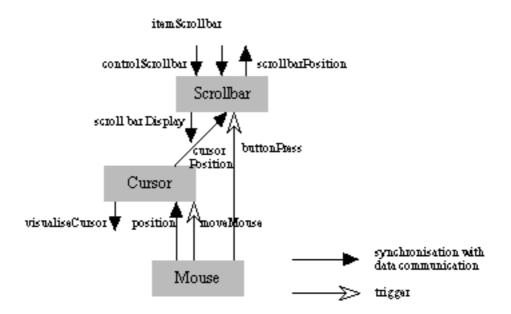
Figure 3.9. Modelling a scrollbar with the Pisa interactor (adapted from [150]).
