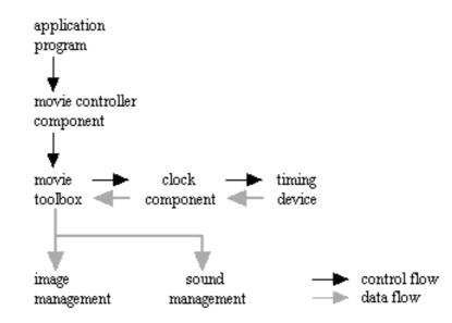
Figure 5.1. Relationships of an application, the movie controller component, the Movie Toolbox, and a clock component (adapted from [9]).
