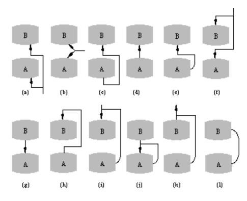
Figure 6.1. The range of connection types of ADC interactors. Arrows indicate gates for input or output. The last case represents a simple synchronisation.
