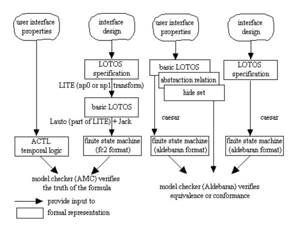
Figure 7.1. Illustration of two possible approaches to model checking of LOTOS specifications. In the left, using the AMC tool and in the right using the Caesar/Aldebaran toolset.
