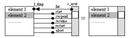
Figure 4.5. A scrollable list as a composition of a list-window and a scrollbar.
