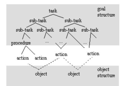
Figure 7.4. The main elements of TKS. Single lines indicate decomposition of task activity. Dashed lines indicate that an action is applied to an object.
