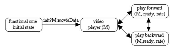
Figure 5.4. The operation of the functional core: Each node is described by a separate process specification. Arrows indicate invocations of a process by another.
