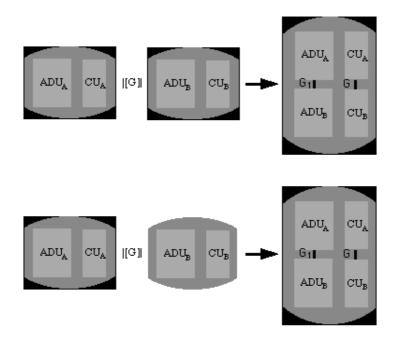
Figure 6.5. Synthesis applied (a) to the synchronous composition of two abstract views, and (b) to the composition of an abstract view and an interactor.
