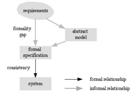
Figure 3.2. Abstract interaction models can help bridge the 'formality gap' between informal requirements and design specifications (adapted from [49])
