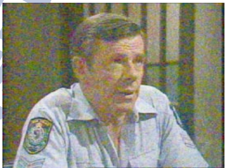
Fig.3: When TV signals are too weak for good reception, this is the kind of picture you get. This is usually described as an image covered in 'snow', or 'coloured pepper and salt'.
