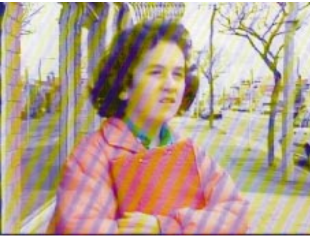
Fig.8: The kind of effect you can get from EMI caused by a continuous radio signal, such as from a radio transmitter or diathermy. The coloured lines can be sloping either way, and at any angle.
