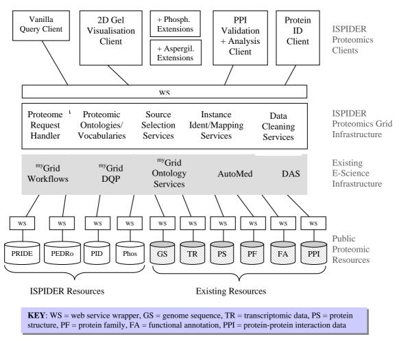
**Figure 1: ISPIDER Architecture**
