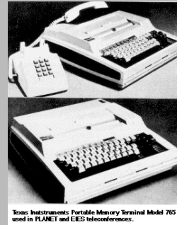
Image Instruments: Portable Memory Terminal Model 765 used in PLANET and EIES teleconferences.
