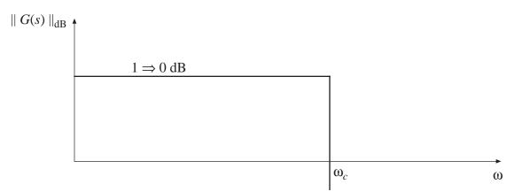
Using the Fourier transform, it can be shown that this transfer function leads to a nonphysical transient response. The output signal must change before the input changes, and the response is not causal. Hence, it is physically impossible to construct a filter having this frequency response.
