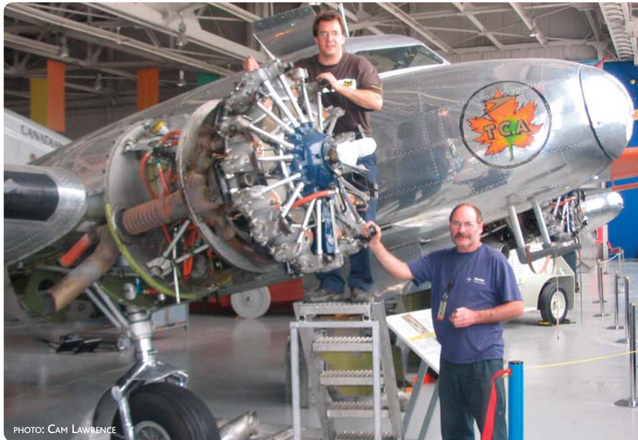
Licensed Aircraft Technicians Mike Clarkson (on the ladder) and George Huntington remove, check, and clean the spark plugs.
