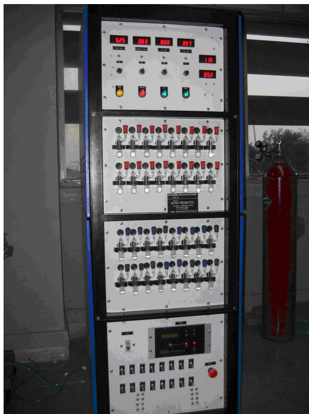
Figure 5.7: Front view of the 4-component gas mixing unit with 16 output channels.
