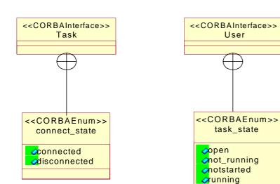
This diagram shows the the definitions of the enums and shows their namespace containment within specific interfaces. Many UML tools do not support UML's namespace containment
