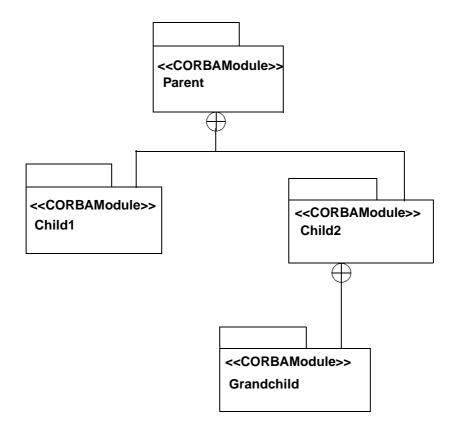
Figure 3-16 Module Namespace Containment Notation
