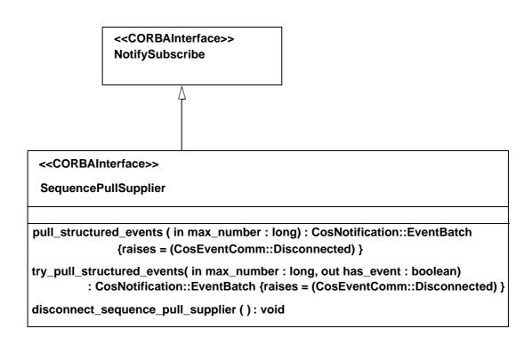
Figure 3-33 Example IDL Interface with Operations
