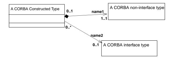
Figure 3-13 Aggregate Notation for CORBA Constructed Types
