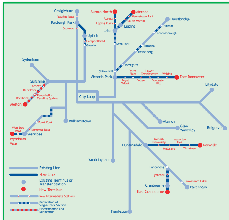
Map 1 Infrastructure expansion on Melbourne's train system: Extensions and additional stations to serve the outer urban growth areas, new lines to East Doncaster and Rowville.
