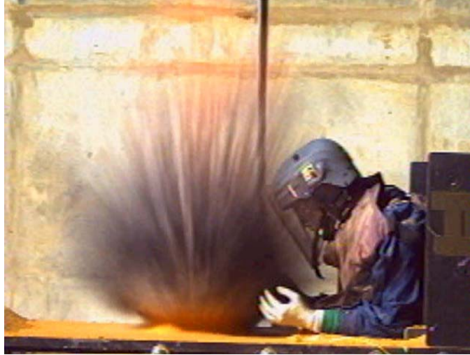
Figure 1: Simulated Antipersonnel Mine Blast with Hybrid III Surrogate
