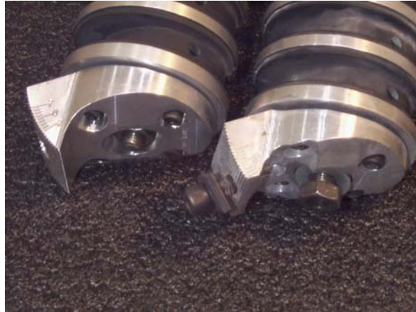
Figure 49: Photograph of Unmodified (Left) and Modified (Right) Dummy Neck Bracket
