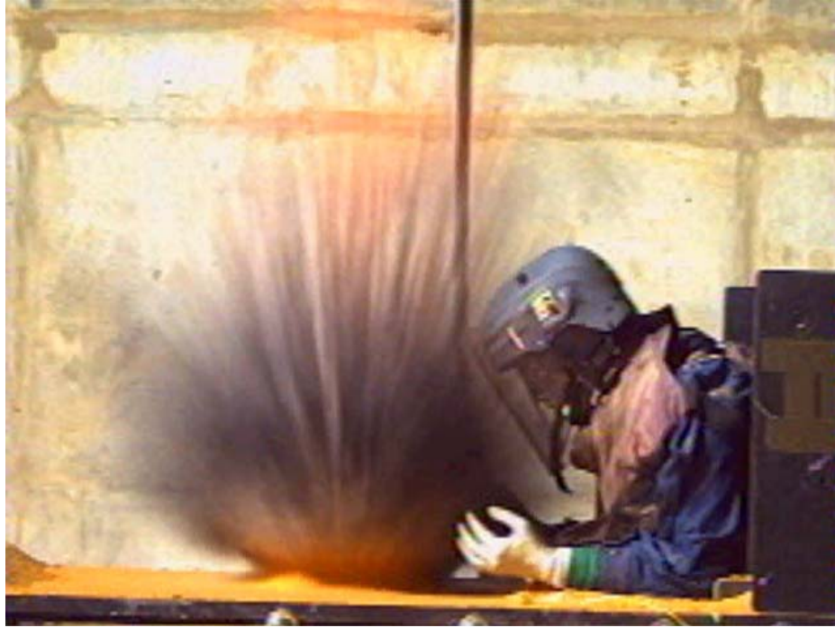
Figure 9: Simulated Antipersonnel Mine Blast with Hybrid III Surrogate
