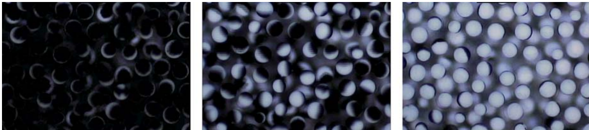
Gyricon - microcapsules switching from dark hemisphere to light.
