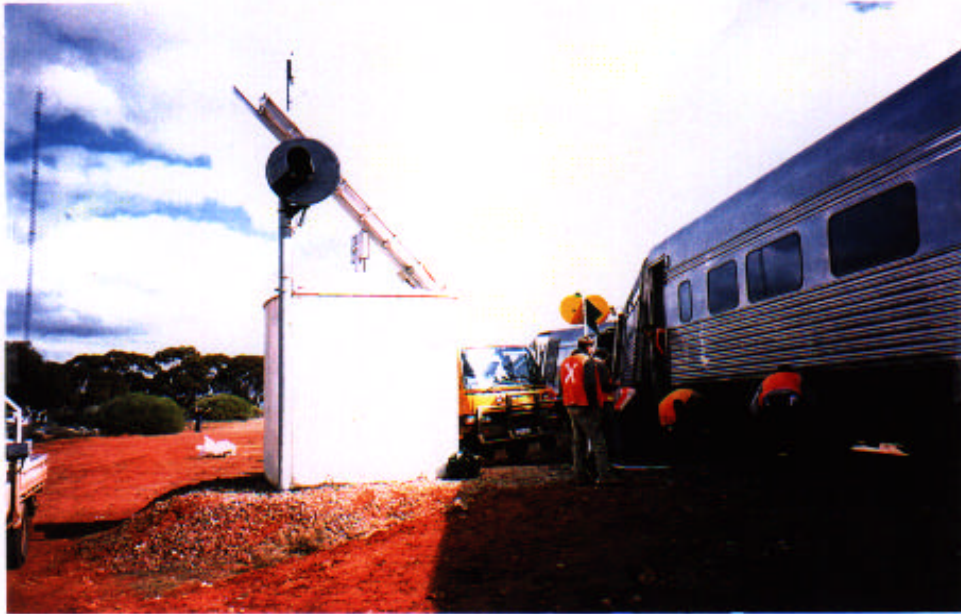
Figure 9: Flashing light indicator and yellow dumb bell showing points set for loop.
