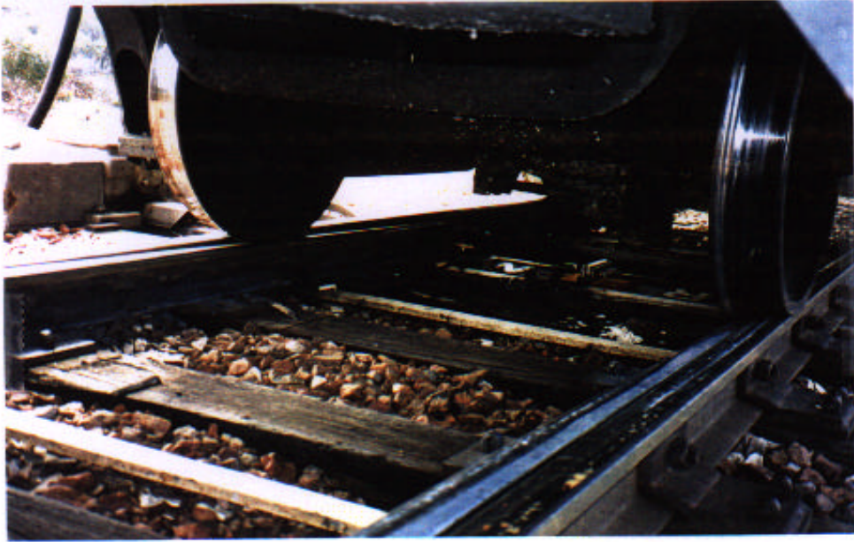
Figure 11: Carriage on points which are clearly set for loop.
