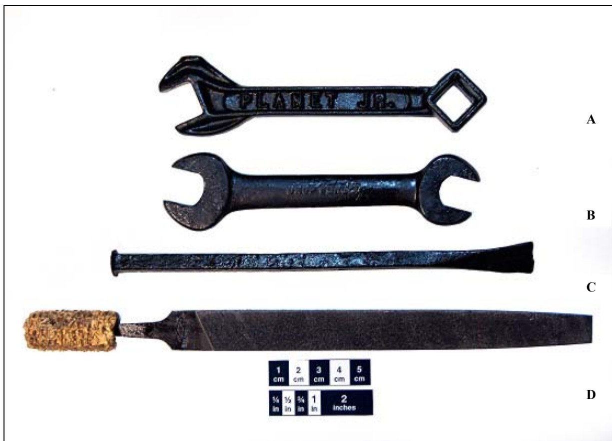
Fig. 9. Tools recovered from house. A, “Planet Jr.” open end and box end wrench; B, Open end wrench; C, Wrought chisel; D, File with corncob handle. Courtesy Morrell and Associates.
