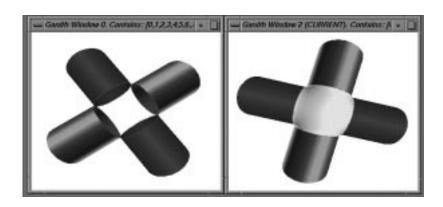
Figure 1. A  $C^1$  Join of Cylinders with a Quartic Surface
