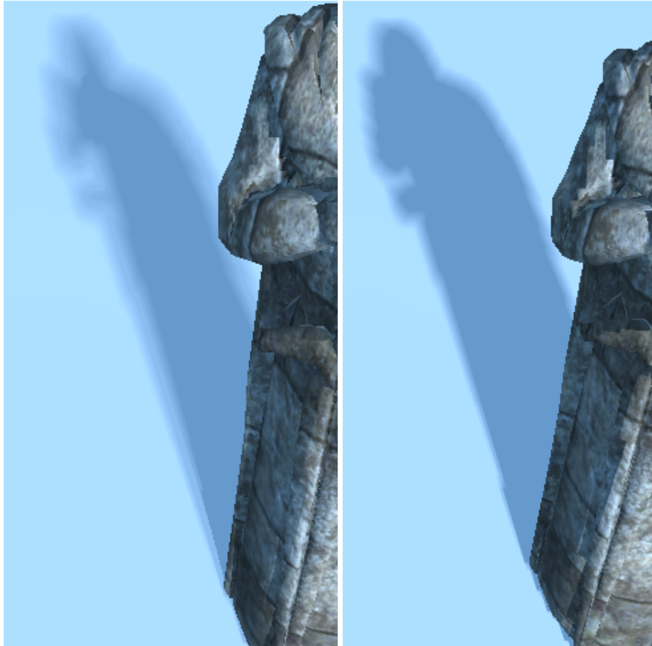
Fig. 10. Visual comparison of our algorithm with smoothies. Shadow map size is 256 \times 256 and the lightsource r = 12 . (a) Our algorithm (b) smoothies. Notice how with our approach, the umbra shrinks and has disappeared almost completely at the head's shadow. Model courtesy of Playlogic Game Factory BV, copyright 2004.
