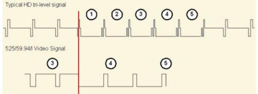
With vertical timing issues now resolved, you may find that standard definition sources converted to HD, or HD sources converted to HD-SDI with A/D converters fall outside of the auto-timing window of your production switcher or HD Master Control. The use of separate black or tri-level reference signal segments will provide a means to steer these problem devices so that they fall within available timing window.
