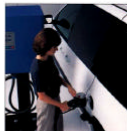
▲ Right where it should be, the charging point is located in the same location as the fuel fill on a gasoline-powered minivan.
