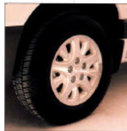
▲ Low rolling resistance tires reduce road friction.
