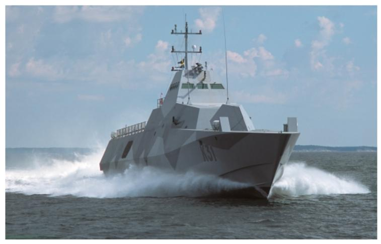
hoods. All other noise-generating equipment such as pumps and fans are mounted to damp out their natural vibration. Air intakes and exhausts are designed for minimal flow noise. Fluid-filled pipes are insulated. The hull material is nonmagnetic, and standard equipment components, where feasible, are selected for their non-magnetic characteristics. An on-board degausser takes care of exceptions.
