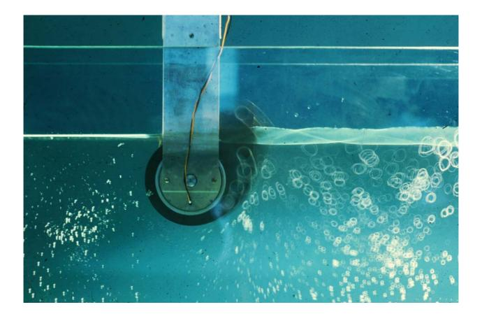
This photograph, taken by Jamie Taylor in 1976, is a one-second exposure of a duck model on a fixed mounting in a narrow tank. The orange and black wires are part of an electromagnetic dynamometer, which is absorbing power. Waves are approaching from the right. Drops of a neutrally buoyant tracer-fluid consisting of a mixture of carbon tetrachloride and xylene with titanium oxide pigment have been injected to show the decaying orbits of wave motion.
