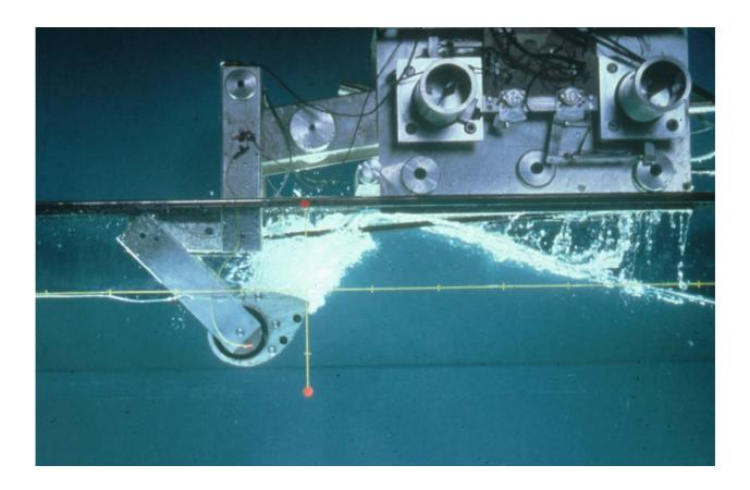
This photograph, from 1977, shows the second model mounting used for simulating the behaviour of long spines in a narrow tank and for survival tests. The vertical and horizontal movements of the rig are force-sensitive and can be given separate stiffness, damping and inertia. The electronic control can also allow them to be programmed to yield at a chosen force.
