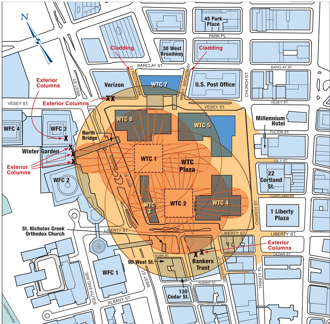
Figure 1-7 Schematic depiction of areas of collapse debris impact, based on aerial photographs and documented damage. Striped areas indicate predominant locations of exterior steel columns. Inner circles indicate approximate radius of exterior steel columns and other heavy debris. Outer circles indicate approximate radius of aluminum cladding and other lighter debris. Heavy Xs show where exterior steel columns were found outside the predominate debris areas.
