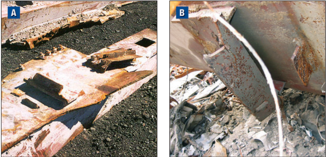
Figure B-9 (A) Visco-elastic damper angles bolted to angle welded to spandrel plate and (B) failed bearing seat connection.
