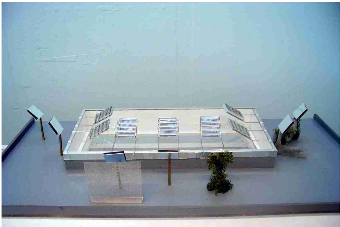
Figure 7: picture of the scale model of the Heliostat systems with redirecting mirrors on the roof
