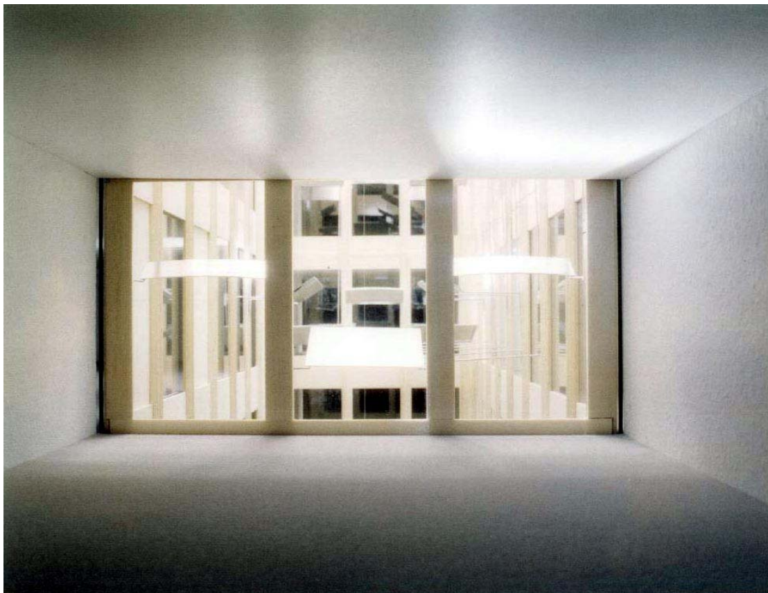
Figure 5: pictures of the scale model of the inner courtyard with redirecting mirrors
