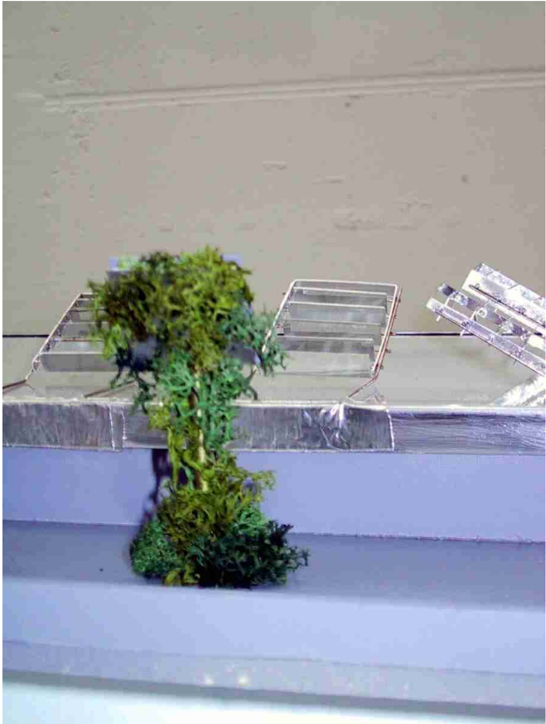
Figure 8: picture of the scale model of the Heliostat systems with redirecting mirrors on the roof
