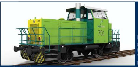
Two-axle Diesel-hydraulic locomotive for shunting service at NS Reizigers B.V.
