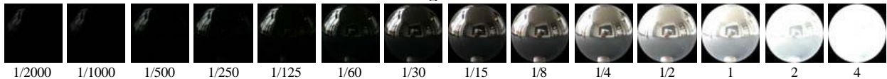
The full exposure range of photographs of the reflective sphere in the lobby
