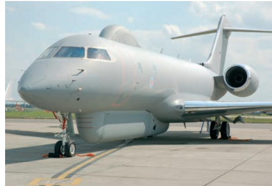
In service since the early 1990s, the USAF's JSTARS fleet ( left ) relies on Boeing's venerable 707 airframe. The Sentinel ( above ) is a heavily modified Bombardier Global Express business jet
