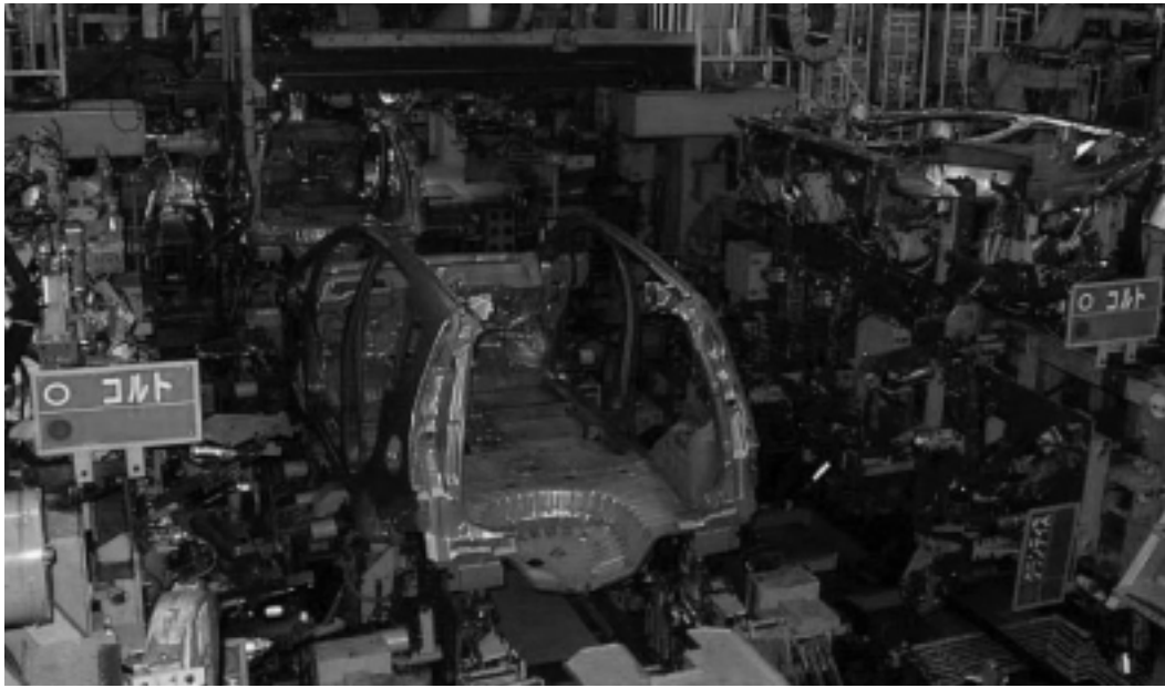
Fig. 6 Flexible welding line using four-face rotatable fixture
