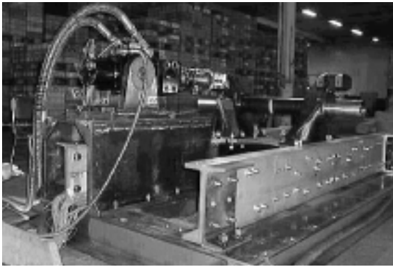
Fig. 10 Strength test of aluminum frame
