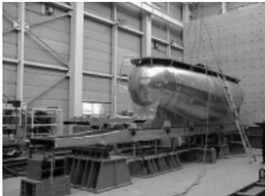
Fig. 6 Stiffness test of aluminum frame
