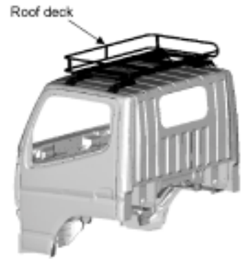
Fig. 14 Roof deck installation
