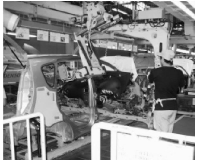
Fig. 9 Installation of instrument-panel module
