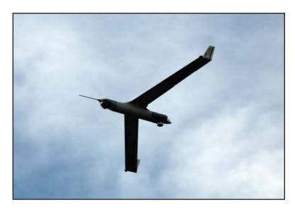
**ScanEagle<sup>TM</sup>** delivers an unmatched combination of endurance, low cost, utility, and small operational footprint. Able to fly for over 15 hours, the ScanEagle A-15 is composed of 5 major modules that are all field replaceable: the nose, fuselage, avionics, wings, and propulsion. The standard payload, housed in the nose, can also be swapped in the field in only a few minutes for a wide variety of sensors available through Insitu.
