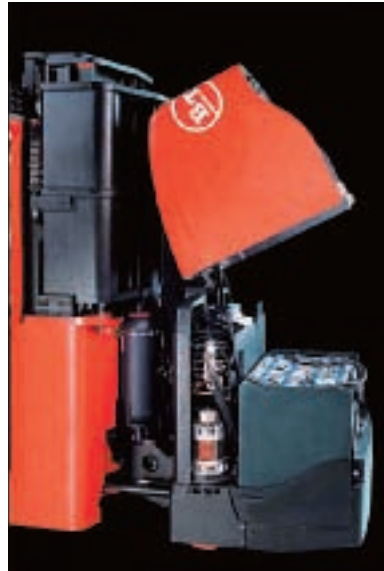
Since the motor is smaller, its requirements for battery power are also smaller, which in turn translates into longer operating hours per charge.
