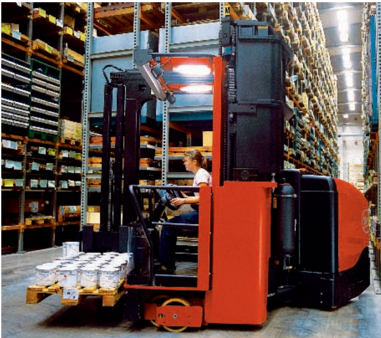
Despite its size, the C15 requires less space in the warehouse to maneuver thanks to its articulated steering.
