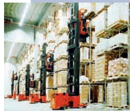
The driver can raise himself to the racks to examine or break up pallets.
