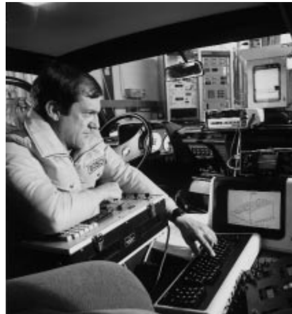
The technical centre at Schwieberdingen near Stuttgart was and is the "Think Tank" for the further development of modern engine control units. The photo shows the digital Engine Control Unit being matched to a specific car model for a test run.
