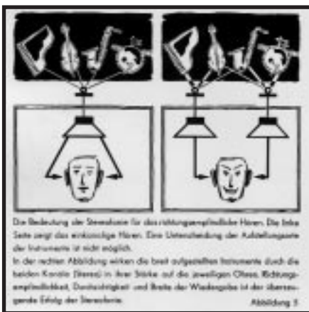
Blaupunkt drawing of 1960. It demonstrates to the reader how stereophony works.
