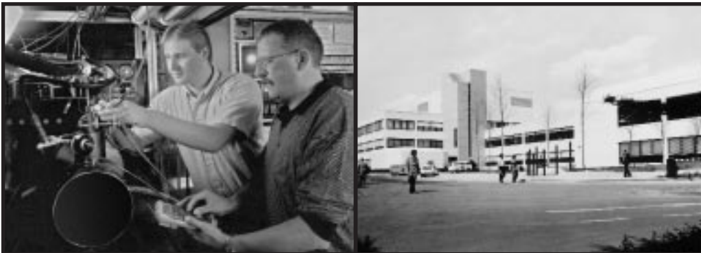
Photo left: Two staff members preparing an exhaust-gas test on a diesel engine on the Feuerbach engine-testing field, 2000
