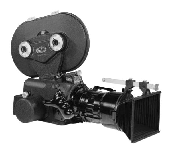
ARRIFLEX 35 BL is the first self-blimped "studio-silent" camera. Compared to the 35 - 50 kg which a camera weighs together with a separate blimp, this 35BL camera weighs only approx. 15 kg. Put to the test the first time under extreme conditions at the Munich Olympics, it proves itself perfectly. More than 1700 cameras of this type are sold.
