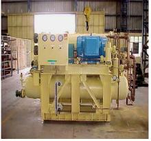
in commission, R-12 AC and Ref plants are being replaced with indigenous plants using lesser depleting R-22 gas. This replacement is being undertaken on ships in a phased manner. All new construction projects and ships undergoing Mid Life Update (MLU) are being fitted with plants using R-134A, a non-CFC refrigerant.
