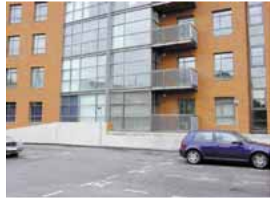
The consequence of failing to consider the relationships between outdoor and indoor space. Here car parking on a raised deck compromises the privacy (and potentially the security) of first floor apartments resulting in permanently drawn blinds. Deansgate Quay, Manchester
