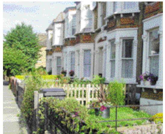
A small front garden (within a 3 – 5 metre setback) provides privacy and a buffer to the street. Stanstead Road, Lewisham
