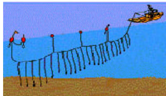
Longlining equipment involves long stretches of line set with thousands of baited hooks. Credit: New Zealand Seafood Industry Council
