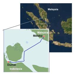
The project, a full turn-key repeaterless system spanning 150 kilometers connecting Dumai (Indonesia) and Melaka (Malaysia), has been completed in six months and is initially equipped to transmit a capacity of 20 Gbps and upgradeable up to 320 Gbps.
