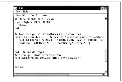
Figure 148. Init Routine Code to Load ListBox Object
