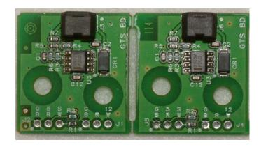
The Gear Tooth Sensors (GTS) should be wired to the Robot Controller's (RC) digital interrupt inputs. The boards require both a +12 volts supply and a +5 volt supply, which is labeled on the boards. The current draw for these sensors is relatively low at 16mA.
