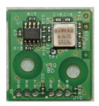
The Yaw Rate Gyro (YRG) should be connected to two of the RC analog inputs. Please note that the output labeled "T" is for "Twist" or rotational velocity. The output labeled "R" is "Relative Temperature". For detailed operation of the Analog Devices ADXRS150 YRG, refer to the www.analog.com website.
