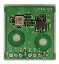
The Dual-Axis Accelerometer (DAA) should be connected to two of the RC analog inputs to measure X-axis and Y-axis acceleration. It will also detect the acceleration due to gravity, and can therefore be used as a static orientation sensor.
