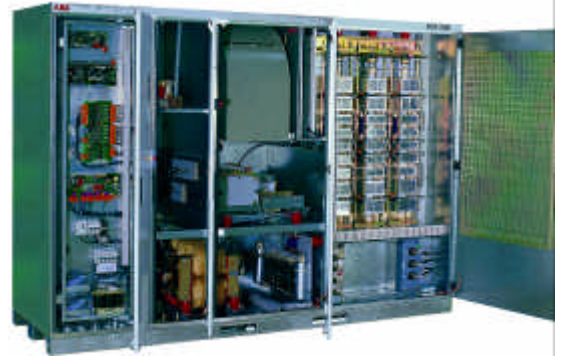
Fig. 11: Air-cooled drive converter of the ACS1000 series (4.16 kV, 1.2 MW sinusoidal output)
