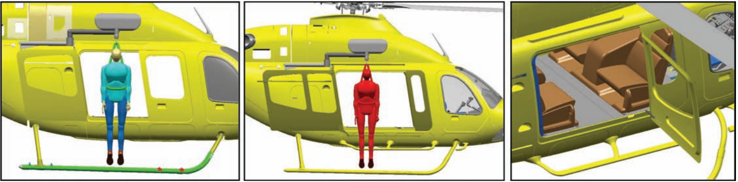
Several door configurations are available on the 429: A basic aircraft sliding door and forward hinged door, left, an optional larger sliding door and a smaller forward hinged door, center, and an optional larger hinged door hinged on the smaller forward hinged door.
