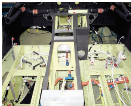
Harness routing, heating system, control fit check and installation.
