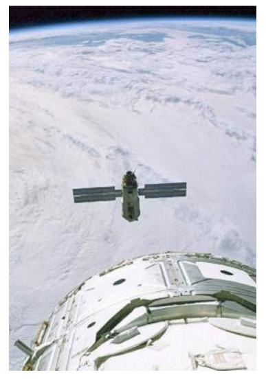
The Zarya control module seen from the Shuttle Endeavour in December 1998 prior to attachment to the Unity connecting module. Launched from Russia, Zarya provides early propulsion and power for the International Space Station.
