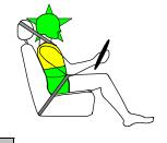
Above: driver injury risks in 50km/h side impact with head protection in pole test
