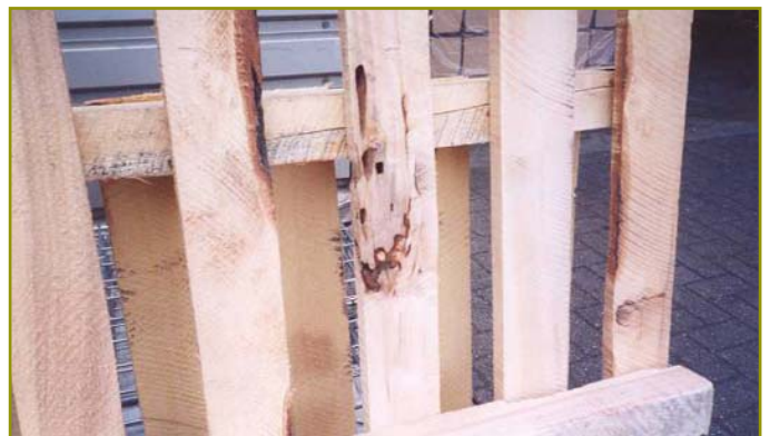
Damage inflicted to wooden pallet.
